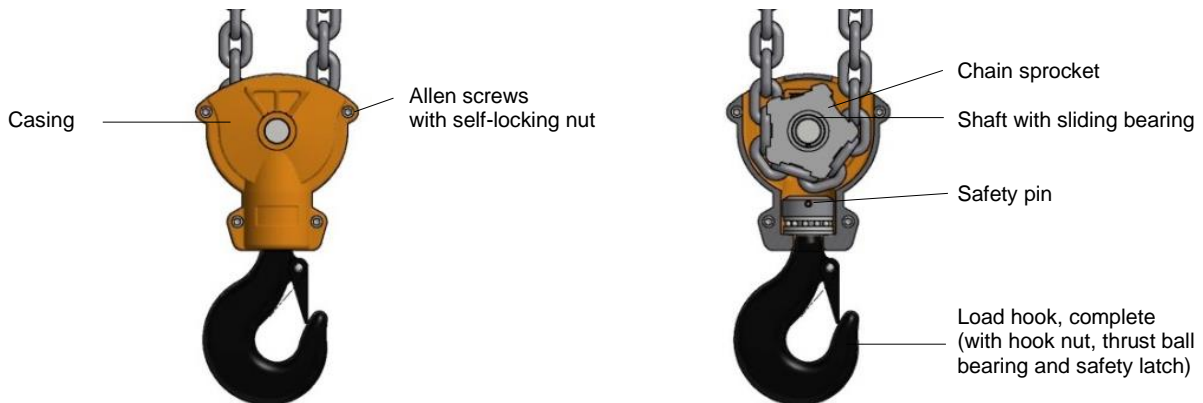
Diagram No 5: Hook block assembly
