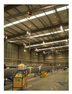
Pacific Hoists were also asked to provide Southern Spars with the facility of being able to operate the hoists either on a individual basis or synchronously in conjunction with any of the five hoists in each production line.
