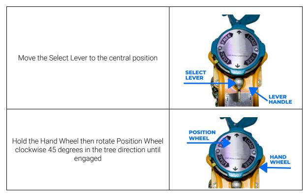
To operate the Lever Block in raise or lower mode:
