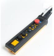
The F-control consists of unbreakable synthetic material resistant to ambient influences. The ergonomically designed housing ensures ease of handling. Up to 18 different control functions can be integrated into a single pendant control; for example key switch, double stage travelling speed and simultaneous control of several motors. The F-control can also be delivered with optional infinitely variable control of hoisting and travelling speeds.
